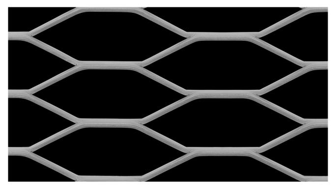
LW Pitch:121.92mmStrand Width:3.50mmSW Pitch:31.65mmThickness:3.00mmWeight:5.29 kg / m2Open Area:78%
